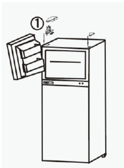
Place the freezer door on the middle hinge. Ensure that the door is aligned horizontally and vertically, and that the gasket seals on all sides before attaching the top hinge. Attach the top hinge and replace the hinge cover.
