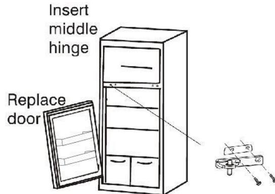
Place the refrigerator door on the bottom left hinge. Ensure the door is aligned horizontally and vertically. Attach middle hinge to top (left) of refrigerator door, attach washer to the back of hinge, align with holes and affix to middle beam with reserved screws. Fasten with screwdriver (not included).
