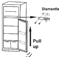
Unscrew and remove the middle hinge and middle hinge washer. Reserve the screws. Lift the refrigerator door up and away from the appliance.
