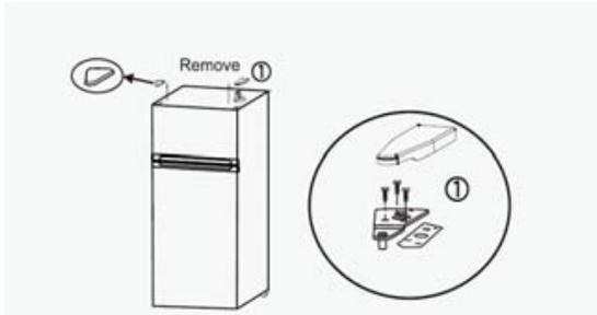
Remove top hinge cover. Unscrew and remove the top hinge and top hinge washer. Reserve the screws.
