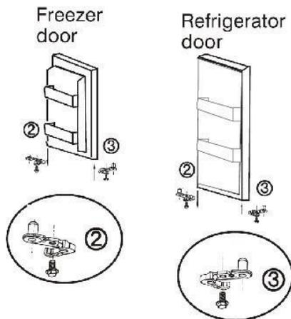
Remove right pin assemblies from the bottom of the freezer and refrigerator doors. On the opposite side, attach the replacement pin assemblies (located in the plastic bag with the Use and Care Manual) with a screwdriver. Note: You must re-use the screws from the pin assemblies that are removed in this step when attaching the new assemblies.
